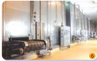
Fully welded stainless steel wall panel enclosure
